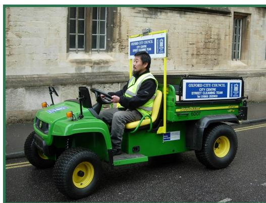
Taking a daily, circular route around 10 city centre streets, the vehicle is 100% environmentally friendly, being powered by electric batteries with no local emissions. As a support vehicle, it is able to service litterbins, collect cardboard and respond to any spillages.
